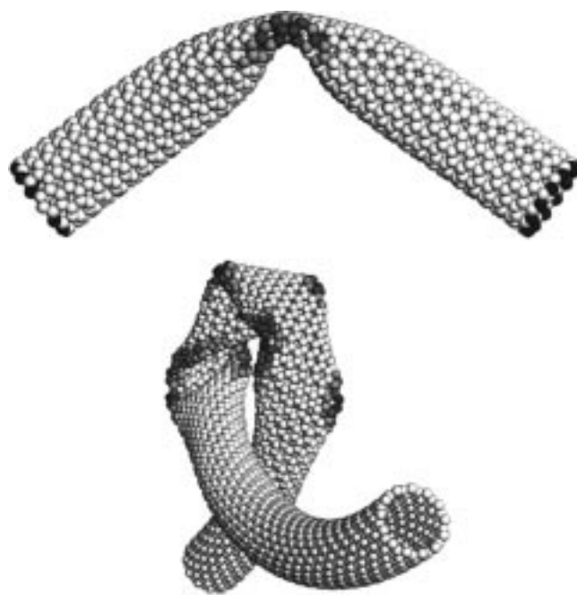
Figure 11. Simulations showing two possible ways nanotubes can deform when they are loaded. The modes reflect the highly elastic nature of nanotubes (Courtesy, Dr. B. I. Yakabson). Details of the deformation mechanisms are reported in Yakabson, B. I.; Brabec, C. J.; Bernholc, J. Phys. Rev. Lett. 1996 , 76 , 2511.
